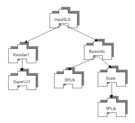
Figure 8. A small LSA session; arrows show the flow of a sparse linear system from input to various solvers.
