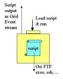
Figure 3. Scriptable Application Manager. (Control Port not shown).
